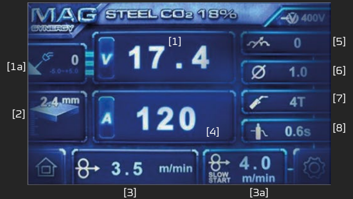
Setting of welding parameters
